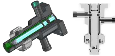
Unique Storage Chamber with Thorough Cleaning Technology, Wiper Ring with Backup seal for harsh media.
